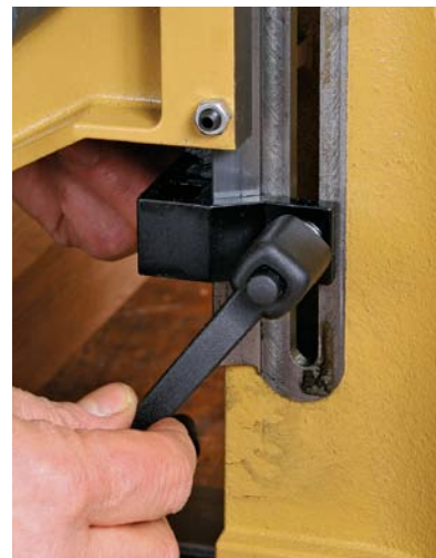
Easy stop. A ratchet handle tightens the Powermatic's stop against the dovetailed ways. It was easy to adjust and tighten.
