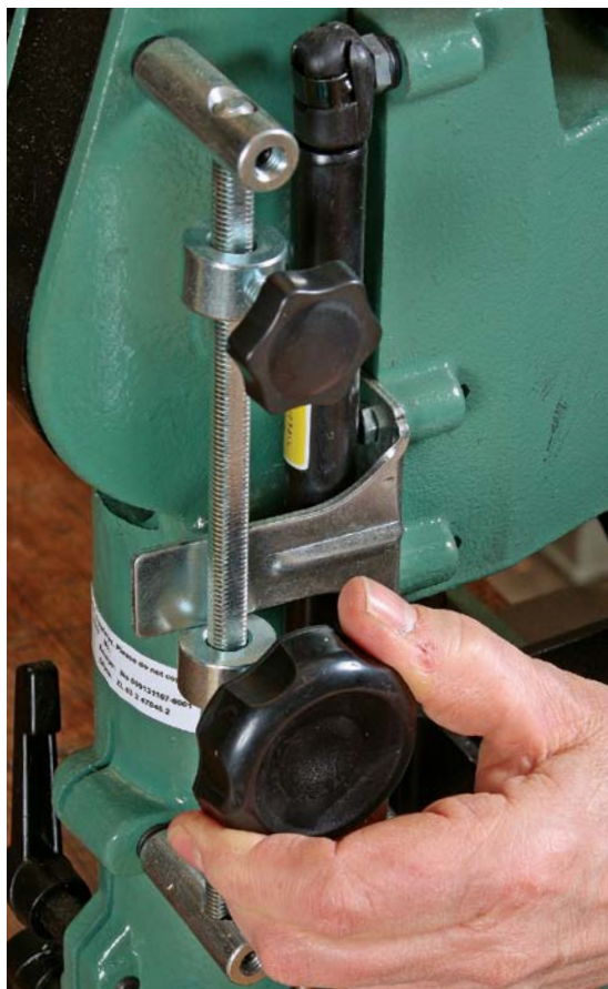
Two stops in one. The bottom stop controls the depth of cut, and the top one allows this chisel to clear the part without having to raise the lever fully—a convenience featured only on the General International 75-050T.
