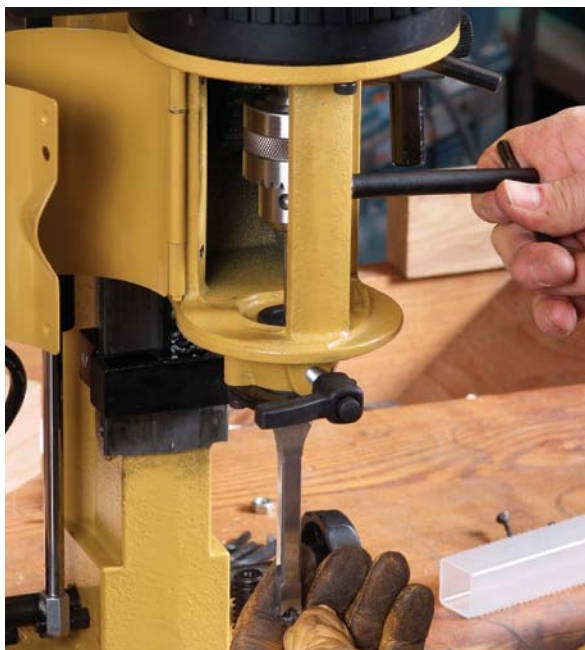
Wide open for business. The door on the Powermatic is the largest and easiest to open. This makes it very easy to lock bits in the chuck.
