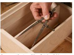
**Compare the two sides.** Set the dividers to one side of the opening. Now check the other side of the opening. It's a quick way to make sure things are correct just before, or during, a glue-up.
