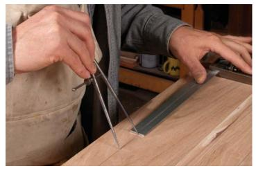
**Line 'em up.** Use a combination square to locate the first hole. With the dividers set at your desired spacing, step off the length of the board. Pushing the tips into the wood gives your drill a solid starting point.
