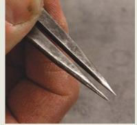
**Make a point.** Latta uses a belt sander and a light touch to sharpen the points on an old pair of dividers. Equipped with a nice set of fine points, your dividers can easily be placed right on the mark, making very fine divots for exact measurements.
