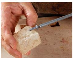
Make a screw shed glue. Heat another screw, the same size as the filed one, with a match (top). Rub it on a block of wax (bottom) to coat the threads, shaft, and underside of the head.
