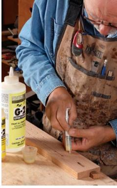
**Fill the hole.** The grain will soak up the epoxy, which is exactly what you want.
