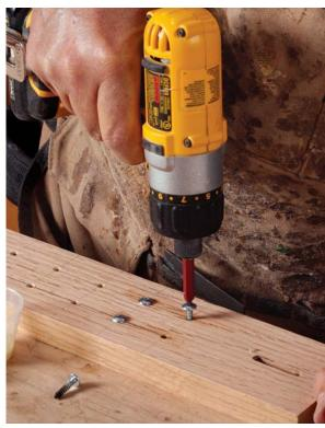
**Create the threads.** Drive in the waxed screw to form durable, reusable threads in the epoxied hole. Remove the screw after the epoxy has cured.
