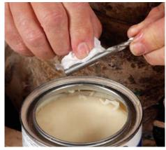
Wax a drill bit. The shank diameter should match the diameter of the jig's holes.
