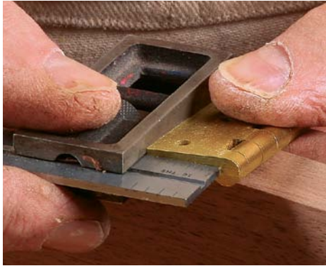
Measure the backset. Set the blade of a square to reach from the back edge of the leaf to the inside edge of the hinge pin.
