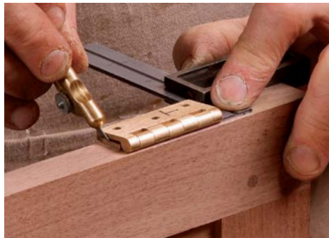
A trick for the other edge. Without moving your square, set the hinge against it, and place the knife tight against the far end (left). Now, without moving the knife, remove the hinge, slide the square against the knife, and mark the line (right) for the other edge of the mortise.
