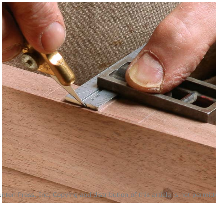
Now the back. Without changing the setting on the square, scribe the line along the back of the hinge.
