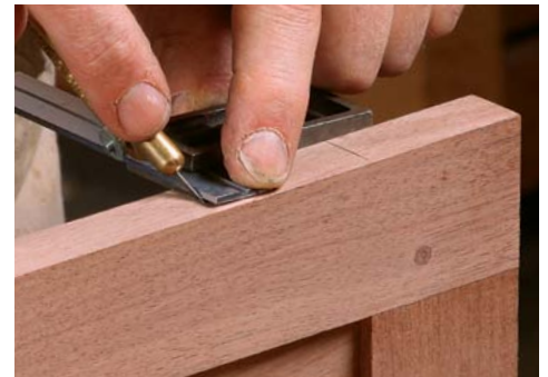
A trick for the other edge. Without moving your square, set the hinge against it, and place the knife tight against the far end (left). Now, without moving the knife, remove the hinge, slide the square against the knife, and mark the line (right) for the other edge of the mortise.
