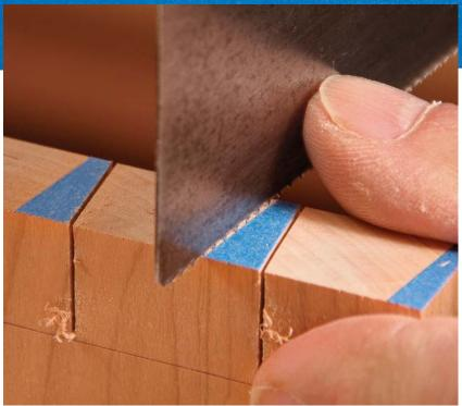
**Use the tape as a saw guide.** Align the saw along the edge of the tape and take light cuts until the kerf is established. As long as you don't cut into the tape, you shouldn't have gaps in your dovetails.
