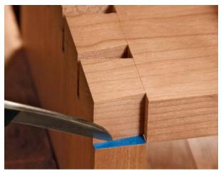
**Transfer the tails.** Apply enough pressure to cut a scribe line through the tape and into the end grain (above). The scribe line acts as a visual reference in case the tape comes off and provides a precise line to pare to during fitting. Then remove the "waste" tape (right).
