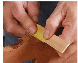
Clean up with sandpaper. A spindle sander makes quick work of the wide curves (above), but to get into the tight corners and work the straight sections of the edge, use a piece of sandpaper wrapped around a thin piece of wood (left).
