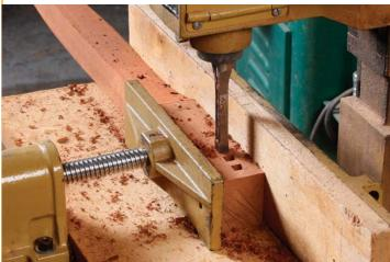
How to set up a mortise when the tenons are cut already. Place the leg and apron between the clamp and fence, with their outside faces against the fence. Adjust the fence so that the chisel aligns with the tenon (top). Set the chisel's cut depth, and cut the mortise (bottom).
