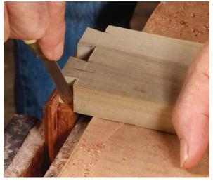
**Lipped front helps with the dovetails.** Push the tails against the lip and then transfer the pin locations to the drawer front.
