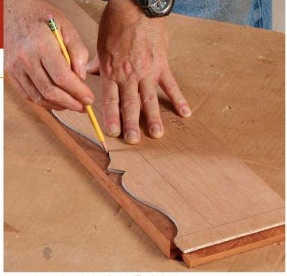
**Lay out the scalloped edge.** To simplify aligning the pattern on the apron, Arceneaux makes it the same width as the apron, and marks the tenon shoulders on it.
