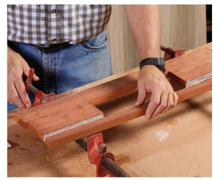
**Glue the apron back together.** Leave out the drawer front to create a front apron with an opening for the drawer. Move the two middle pieces inward to accommodate the drawer's lipped edges.
