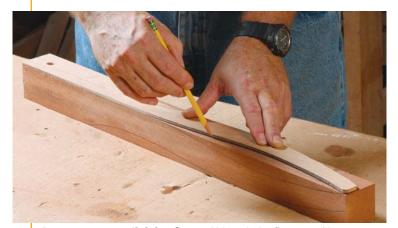
**Lay out on two adjoining faces.** Although the first cut will remove most of the layout lines on the second face, what's left makes it easier to align the template to lay out the pattern for the second pair of cuts.
