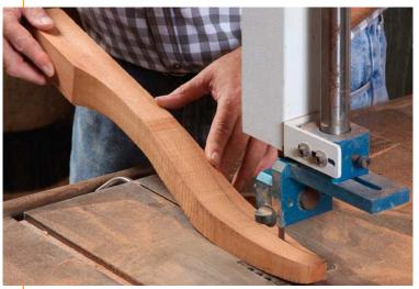
**The second face is tricky.** You must keep the leg in contact with the table where the blade is cutting.
