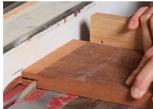
**Two-step tenons.** Cut both cheeks at once with a tenoning jig and the outside blades from a dado set (left). A spacer between the blades determines the tenon's thickness (see below). This setup also cuts the shoulder on the apron's back. Cut the front shoulder at the tablesaw (above), using a miter gauge. Cut the top and bottom shoulders that way, too.
