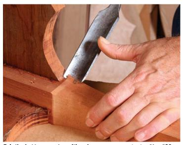
Fair the leg-to-apron transition. Arceneaux uses a gouge with a #30 sweep, and then sands the transition up to P220-grit.
