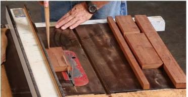
**Cut the drawer front from the apron.** After ripping the blank into three strips, cut the middle strip into three pieces. The center piece becomes the drawer front, and the outer pieces are ripped narrower.
