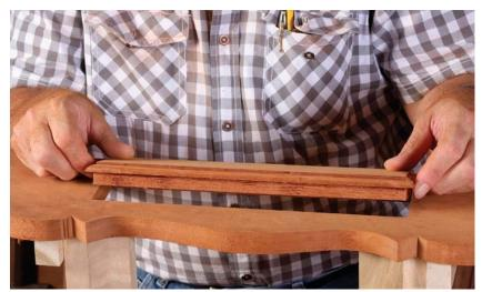
**Test the fit.** The top and bottom rabbets are the most critical, because the front will expand the most across the wood's width. Leave plenty of room to accommodate seasonal changes.
