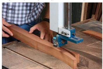
**Cut the first face.** Both of these cuts are easy, because you have a flat reference surface to set down on the table.
