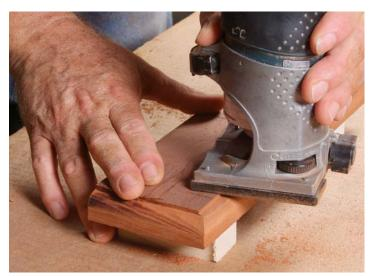
First profile the drawer front. Two scraps beneath the front create enough clearance to prevent the bit from contacting your bench.
