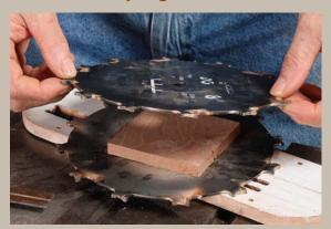
Mill a spacer so that its thickness matches the width of the mortising chisel. Place it between the two outside blades of a dado set (above), orienting the blades so that the high points of the teeth face inward. Assemble the sandwich and doublecheck the space between teeth (right).
