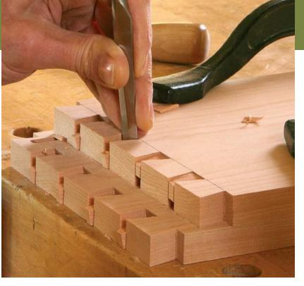
still a wedge, and too heavy a hit will widen the scribe line in both directions. Go up the stairs, making light hits on all the pin sockets. Then, with a narrower chisel, held horizontally with the bevel up, hit into the end grain to remove a chip of waste about  $\frac{1}{16}$  in. thick. This will leave you a nice, square shoulder directly on the scribe line.
