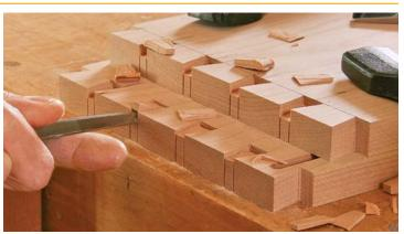
**Halfway home.** Remove the thick waste chips (above) and then resume chopping with the chisel angled. Continue chopping to the halfway point in the board's thickness.
