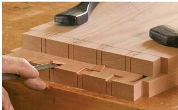
**Pop out a slim chip.** After lightly chopping all the pin sockets, use a narrower chisel to remove the top layer of waste wood with a tap into the end grain. The shoulder should now be about  $\frac{1}{16}$  in. high.
