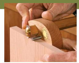
**Set the gauge.** Adjust the marking gauge so its cutter just overhangs the pin board (above). The overhang will produce dovetails that are slightly proud. Scribe the baseline across both faces of the tail boards (right).
