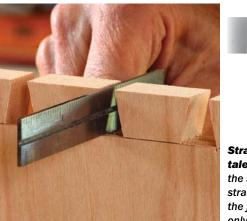
1 2 Undercutting ensures tight fit at outside edges.
