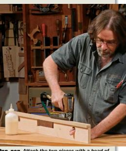
**Pop, pop.** Attach the two pieces with a bead of glue and a few nails (or countersunk screws).
