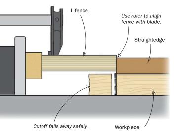
**Rip it flush.** Push the workpiece through, letting the template bear against the L-fence. The beauty of the L-fence is that if you bobble the workpiece, you're cutting into the waste, not the work. If you make a mistake, just run it again.
