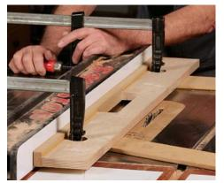
**Set it straight.** Set the L-fence  $\frac{1}{46}$  in. to  $\frac{1}{8}$  in. above the blades. Shims hold the fence parallel to the table while you tighten the clamps.
