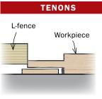
**Tenons, too.** After the cheek cuts, cut the shoulders with the tenon riding against the L-fence. The cutoff falls away safely.
