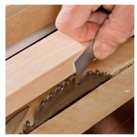
allows the offcuts to drop away harmlessly. To cut a rabbet, raise the dado blades up to the depth of the rabbet and clamp the L-fence to the rip fence, positioning it <sup>1</sup>/<sub>16</sub> in. above the blade, parallel to the table. As with a sacrificial fence, the width of the exposed blades equals the width of the rabbet. But unlike a sacrificial fence, the L-fence doesn't need to be replaced.
