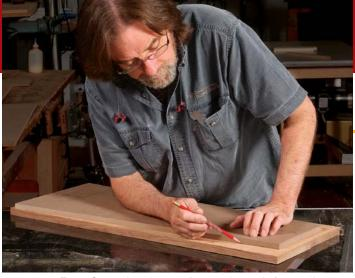
**Trace it out.** Lay the template on the workpiece and trace around it. Plywood and MDF make better templates because their dimensions stay stable over time.
