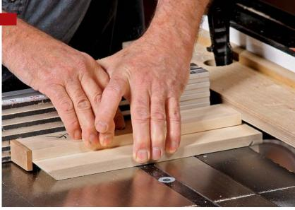
**Get the hook.** With the L-fence set for a mitered flush cut (see opposite page), use the gauge hook to make the second miter. Use the miter gauge and let the end of the gauge hook ride the L-fence.
