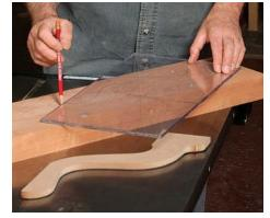
**Two templates.** Trace the leg pattern onto a square Lexan template. Then use the clear template to locate a leg on the blank and mark the straight edges.
