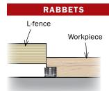
**Run your rabbets.** Keep the edge of the workpiece tight against the edge of the *L*-fence as you make the cut.
