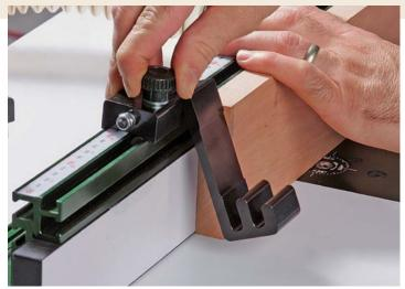
**Use the track on the fence for stops.** The fence is also a good place to attach hold-down-style featherboards and bit guards.
