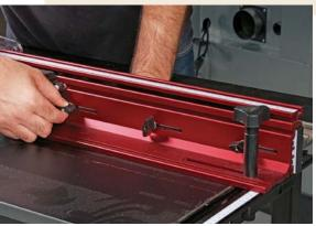
**Slots in the fence for adjustments.** On JessEm's fences, loosening three knobs on the back lets you slide the fence.
