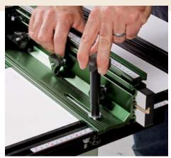
**Lock down to a T-track.** The Excalibur (shown) and JessEm fences slid easily in the T-track, and you don't have to reach down behind the fence to loosen and tighten them.
