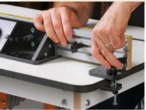
Clamp the table's edge. Only the Woodhaven fence locked down this way, but the lock was easy to use and made it a snap to quickly pull the fence off the table for pattern routing.
