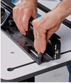
**Through a slot in the table.** Because of this system, the Rockler and Bench Dog fences were more difficult to move forward and back than other fences.
