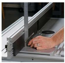
All of the fence faces were square. The T-tracks above them are set back slightly. This decreases the fence's effective height, but eliminates potential problems with aligning the fence face and T-track.
