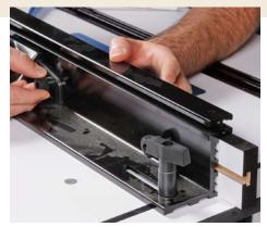
**T-tracks in the fence face work, too.** The only downside is that replacement fences need the T-track, too. That means you need a special router bit. (Rockler's Pro Phenolic table is shown.)
