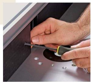
A less convenient approach. The fence on Sommerfeld's table requires the use of an Allen wrench (provided) to loosen screws before the faces can be adjusted.
