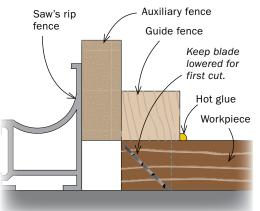
Second pass completes the miter. With the majority of the waste removed, raise the blade and make the final trim cut.
