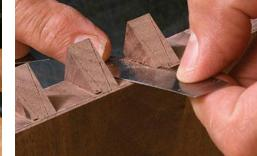
**New dovetail tool: tin snips.** To cut the angled shoulders of the pins, Fortune modifies a \$17 flush-cutting trim saw so it can fit between closely set pairs of pins.
