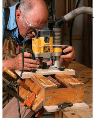
**Hog out the waste.** Lock down the carriage for each pass, staying clear of the knife lines. Cut to full depth with a series of light passes. Then creep up on the lines.
