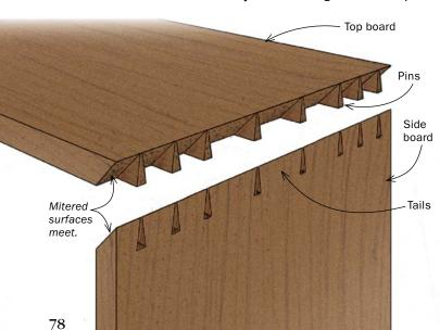
The tails of a half-blind mitered dovetail are cut as normal tails and mitered afterward. The trick to the joint is mitering between the pins.
