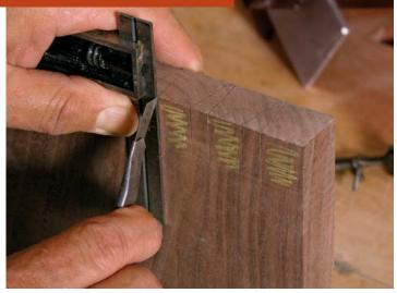
Mark the pins with a knife. Deep layout lines are essential to guide the routing. Don't lay out the miter so it comes to a complete point—leave a  $\frac{1}{32}$  in.-wide flat at the tip to allow for planing and sanding after assembly.
