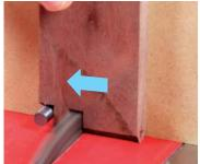
The second leaf is notched on both ends. Use the first leaf as a stop (left). Its edge will align precisely with the edge of the blade's teeth, so the notch you cut is exactly ½ in. wide. With the first notch over the pin, the leaf is properly aligned to cut the second one (above).
