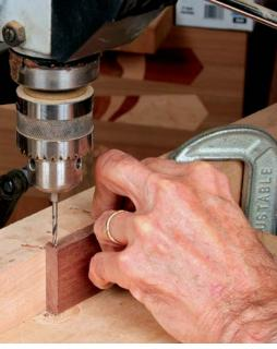
**Check your work.** With the drill press off, flip the piece and lower the bit into the hole. If it enters smoothly, the hole is centered. If not, adjust the fence, cut off the end, and try again.
