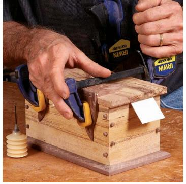
**Business card prevents binding.** Use three cards, one each for the back and sides. Check the lid's overhang on both sides before clamping.
