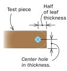
Aim for the center. Do your best to adjust the fence so that the bit is centered on the leaf's thickness, and drill a shallow hole.
