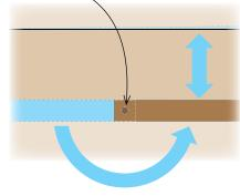
Drill, then flip test piece end for end to test fence placement.
