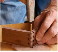
**Knock in the pin.** Put the hinge on a small scrap of plywood with a hole in it. Drive the pin through and a bit proud of the other side.
