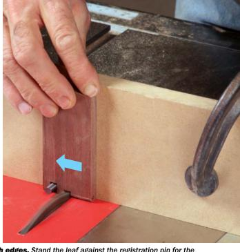
**The first leaf has a knuckle on both edges.** Stand the leaf against the registration pin for the first cut (left). It straddles the pin for the rest of the cuts (right), one notch aligning the leaf for the next one. Hold the top end of the leaf against the jig to keep it from moving.
