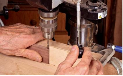
**Drill just past halfway.** Then drill from the other edge. Check that the pin enters smoothly through the completed hole, then drill the real leaves.
