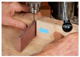
**Stop block steps in.** Insert the bit into the hole, then align the test piece perpendicular to the fence. Clamp a stop block against it. This ensures that the hole is spaced an equal distance from the edge and end of the leaf.
