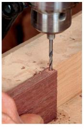
Drill bit should slide in smoothly in both orientations.
