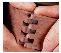
Knuckle sandwich. The knuckles should come together with a bit of resistance, but you should still be able to move the leaves easily.
