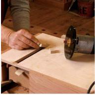
**Spacers control the length.** Graduated drawers require different-length sockets. Use press-fit spacers to control the router's travel.
