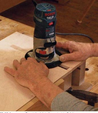
**Multiple passes.** To cut the joints from start to finish without disturbing the drawer front, Turner sets up three routers with different bits. If you don't have extra routers, change bits between cuts and use test cuts in a sample board to reliably reset the depth of cut.
