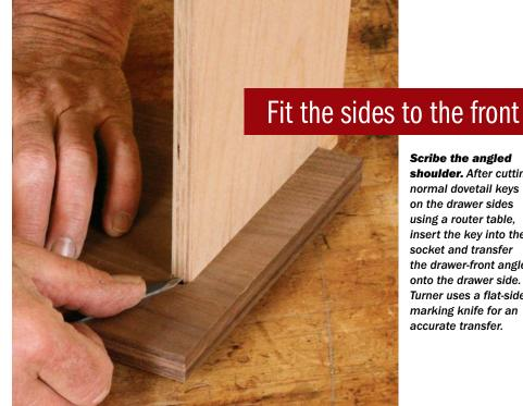
Scribe the angled shoulder. After cutting normal dovetail keys on the drawer sides using a router table, insert the key into the socket and transfer the drawer-front angle onto the drawer side. Turner uses a flat-sided marking knife for an accurate transfer.
