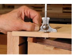
**Precise height is key.** Due to springback, no two bent-laminated drawer fronts are exactly the same. Use paper or card-stock shims to level the drawer fronts.
