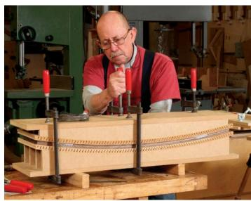
**Create the curve.** After rolling Unibond 800 urea resin glue onto the stack of ½-in.-thick laminates, Turner binds the ends in stretch-wrap to keep them registered. Then he clamps the stack between forms and lets the glue cure overnight.
