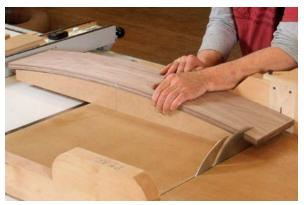
**Cut it to length.** Mark the centerline on the drawer front and align it with the center mark on the cradle.
