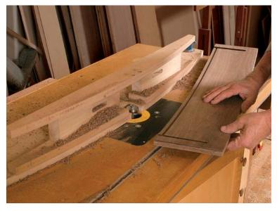
**Curved fence** for a curved groove. To rout the stopped groove in the drawer front that will accept the drawer bottom, use a slot-cutter in the router table. To support the piece, make a fence from male ribs cut to the same radius as the concave side of the drawer front.
