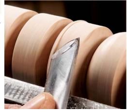
Pivot from the thumb. Use the tool rest as a fulcrum when slicing through the wood. The motion looks and feels like a planing cut in which you ride the bevel. You'll need to move the handle away from the center of the bead to do so.
