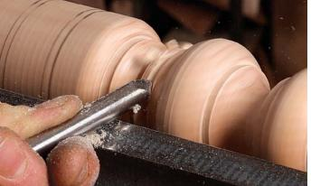
Map out the spindle and excavate. Use two parting-tool cuts to define the shoulders, and the spindle gouge to remove most of the waste in between.
