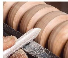
Now the right. To cut a bead with a spindle gouge, enter the cut near the center and simultaneously roll the tool and ride the bevel down the side of the bead.
