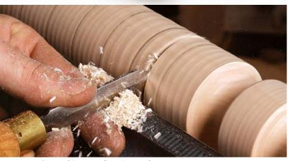
Start with a pencil and a parting tool. Mark pencil lines every 1 in. and make notches between them to roughly 1 in. dia. To use the parting tool, start by riding the bevel and then raise the handle to lower the tip.
