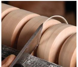
Vertical limit. With each pass, you'll start closer to the center of the bead, and finish with the tool more and more vertical until it's close to 90°.
