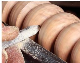
Finish on the side. The gouge will end up tipped all the way onto its side on your final pass.
