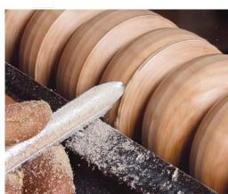
Tricky motion. To keep the cutting edge engaged, you'll need to roll the tool sideways while both lifting the handle and moving it sideways.
