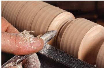
Work toward the pencil lines. Scoop out the sides of the cove. working from side to side to widen and deepen the shape. Continue feeding the cutter forward to raise it out of the cut.
