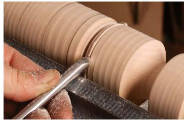
A few small cuts in the middle. Holding the gouge on its side, take shallow cuts on each side of the parting-tool cut. Enter the cut by rolling the gouge back toward level while pushing it forward in a scooping motion. Keep the bevel of the gouge bearing on the wood as you roll and push.
