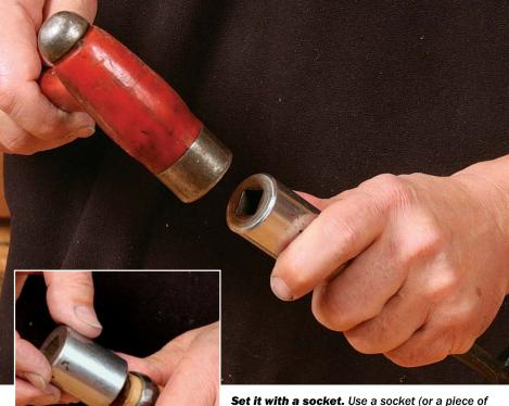
Set it with a socket. Use a socket (or a piece of pipe) just larger than the chisel's handle to direct your hammer blows to the hoop. After the hoop is hammered down, about <sup>1</sup>/16 in. of the handle should be showing above it.
