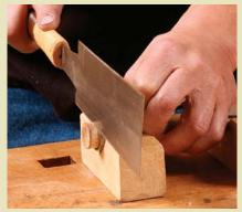
In case it's overlong. If the hoop seats down too far on the handle, you can saw off the end of the handle, leaving <sup>1</sup>/16 in. showing.
