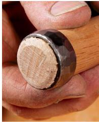
**Make a mushroom.** Use light hammer taps with a pulling motion while gradually turning the chisel to create an even mushroom shape that will hold the hoop securely in place.
