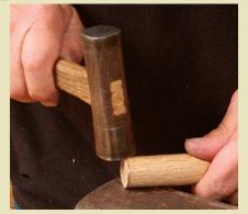
**Hammer, don't file.** If the fit is tight, try hammering lightly with the handle against a hard surface.
