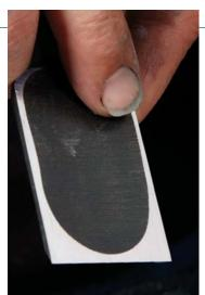
Make it flat around the hollow. The back of the blade is hollowed to make flattening easier. It's critical to flatten the front edge and most of the way up the sides, but not necessarily all the way up the back.
