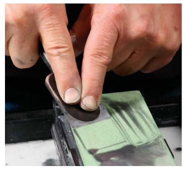
Check the new angle. Because the blade is mostly soft iron, altering the bevel angle on sharpening stones is fairly quick. Fox uses angle blocks to check that his new bevel is accurate.
