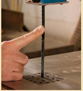
**Two ways to check blade tension.** A simple method is to set the tension one mark higher on the tension scale of your bandsaw (for instance, set it to the  $\frac{1}{2}$ -in. mark for a  $\frac{3}{8}$ -in.-wide blade). You also can check the tension by pressing your finger against the side of the blade (right); if it deflects more than  $\frac{1}{4}$  in., crank up the tension.
