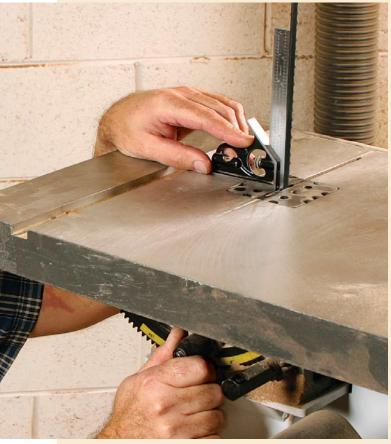
Make sure the blade is perpendicular to the table. Place a square against the side of the blade, and adjust the table until the sawblade is flush against the blade of the square.
