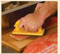
**Joint after each cut.** Run the just-cut face of the workpiece lightly over the jointer (removing about ½4 in. of material) before slicing the next sheet.
