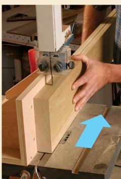
**Pull long stock** through at the end of the cut. Before the board starts to fall off the table on the back side, walk around to the other side of the saw and pull the board through. Support the board with one hand while using the other to hold it flat against the fence. This method also keeps your hands away from the blade.
