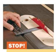
Mark your place before removing the top. Measure the distance between the blade and the left-hand miter slot. Realigning the slot to this measurement during reassembly will ensure that jigs, such as a crosscut sled, will still fit.
