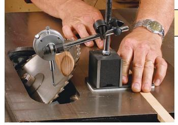
**Check again for parallel.** After bringing the miter-gauge slot parallel with the blade, tilt the blade to 45° and repeat the process.
