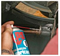
Use a penetrating lubricant on hardto-reach areas. For the worm-gear shafts on the arbor-pivot and -raising assemblies, Johnson uses a penetrating spray that dries quickly.
