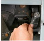
Setting the blade upright. The 90° stop is usually easy to reach. Simply loosen the stop bolt and use a square to set the blade to exactly 90°. Then turn the stop bolt snug to the stop, and tighten the locknut on the stop bolt.
