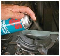
On the worm gears and racks, use a molybdenum-based drying lube. The spray, which withstands heavy pressure, is dense enough to stay in place without running.
