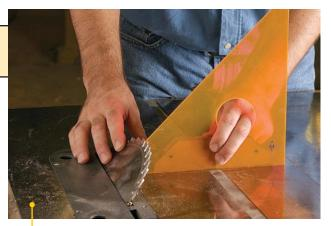
Getting properly inclined. The 45° stop bolt on many saws can't be reached when the arbor is tilted all the way to 45°, so setting it takes some finagling. Loosen the bolt so that the blade stops before 45°. Then tighten it a little, and check the angle with a drafting triangle. Repeat the procedure until you find the exact setting for 45°.
