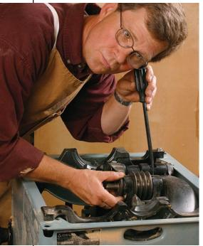
**An old hot-rodder's trick.** A long screwdriver, with the tip held firmly on the bearing housing, makes a good listening device for checking the condition of the bearings.
