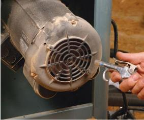
**Remove loose sawdust.** Two good vacuumings, with a blast of compressed air in between, should eliminate loose sawdust inside the cabinet. Clean the motor and/or fan thoroughly with compressed air to ensure cooling efficiency.
