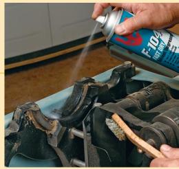
To help remove minor pitch buildup and rid the gears of old grease, use a quick-drying aerosol degreaser and scrub with a wire brush. Surfaces need to be clean and dry before lubricants can adhere well and do their work.
