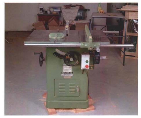
**Top-quality saws cost between \$1,500 and \$2,000.** These saws, what the author describes as Class A machines, have solid cast-iron tables and extension wings and a full-length fence. These heavy-duty, smooth-running machines form the backbone of many small professional and serious amateur woodworking shops.
