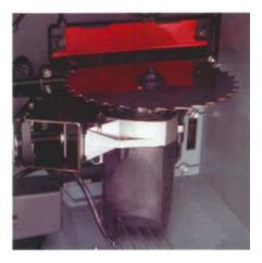
Lightweight tilt and raise mechanisms are typical of low-end saws (above). Less powerful, direct-drive motors also are common in these Class E saws.
