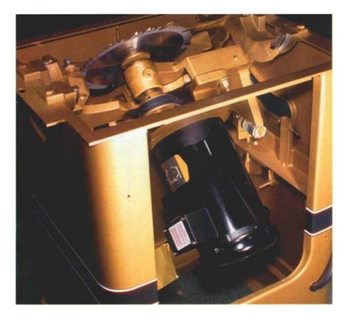
Internal framework is real strength of top-of-the-line saws (left). Heavy-duty trunnions, gears and bearings make for easy adjustments and vibration-free operation in saws costing \$1,500 to \$2,000.
