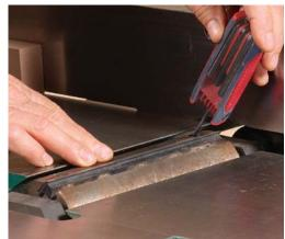
Work to the lines. Start at the same mark to check the height of the other end of the knife (above), adjusting the jackscrews (left) until the board moves the correct distance. Then do the same at both ends of the other knives.
