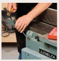
Rotate just a little. Raise or lower a corner of the table by first loosening a set screw and rotating the eccentric bushing with a wrench or screwdriver (above). Use the detents or your own marks as reference (below).
