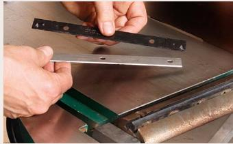
If you don't want to spend time setting knives, disposable blade kits from Esta-USA can be installed and set in minutes. The knives snap into a tabbed holder that sits in the pocket of the cutterhead. The tabs register off the top of the cutterhead so each knife sticks out the same distance. eliminating the need to adjust it. The knives are doubleedged, but can't be sharpened. Kits for an 8-in. jointer with three knives cost \$270 (\$35 for just the knives).
