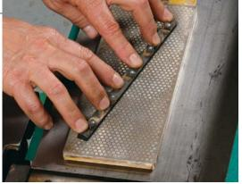
**Flatten the gib.** Use a diamond plate or fine-grit sandpaper stuck to a flat surface to flatten the gib's face and help it grip the knives evenly.
