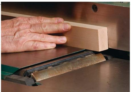
**Work off the outfeed.** With the table raised, use the jackscrews to adjust the height of the knives so that each one just grazes a board when the cutterhead is rotated by hand.
