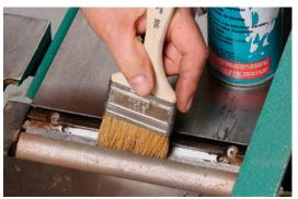
**Brush out the grime.** Use a thick bristle brush and a bit of degreaser to remove caked-on crud that can interfere with setting the knives.
