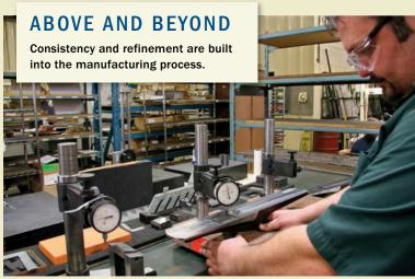
**How flat is that?** Using a dial gauge, machinist Scott Shelley checks the flatness of a jointer plane that he's been milling. Multiple checks are built into the manufacturing process in the Veritas machine shop.
