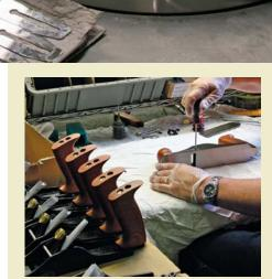
Hand tools hand-assembled. After leaving the machine shop, the tools are assembled, tested for functionality, and inspected for defects before being boxed up and shipped off.
