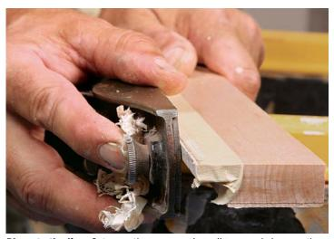
**Plane to the line.** Cut away the excess using a jigsaw and clean up the edge with a block plane.
