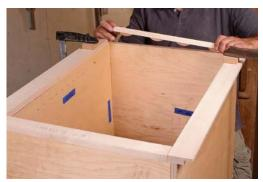
Glue the rails beforehand. Dry-fit the stiles to align and glue the rails in position during assembly. Then remove the stiles so they can be trimmed later.
