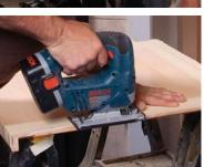
moldings. Instead, I build a quick template from MDF and use it to mark the oversize top so it can be cut to shape perfectly.
