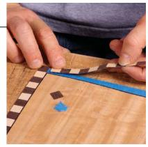
Start at the corners this time. Overlap dark squares at the corners, then simply remove one of them. To get the rest of the banding to fit, trim a bit off a square or two near the center. No one will notice.
