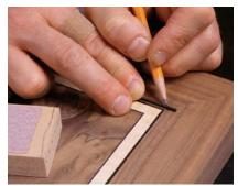
**Pre-fit the pieces.** Mark these at the corner joints (above), using a sanding block or disk sander to make the tiny miters. Thibodeau uses a kids' glue bottle with a narrow tip to inject the glue into the groove, presses in the stringing, and then seats it fully using a small hammer and a wood block (right).
