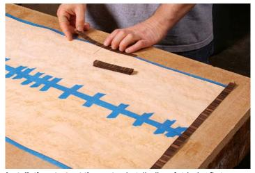
**Installation starts at the center.** Install a line of stringing first, as before. Then mark the center points of each edge, and start adding the crossbanding there, working toward the corners and flipping each opposite piece as you go for a balanced look.
