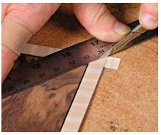
Another angle at the corners. Use a similar technique to make perfect miter joints at the corners, cutting both stringing and banding at once. Line up the straightedge carefully with the corners of the overlap.
