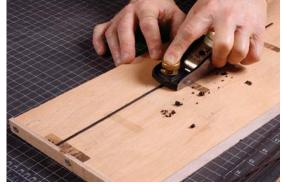
Need to fine-tune it? Make a little planing jig like this one, with a low stop, and add pieces of double-stick tape to keep the stringing from bowing as you plane it.
