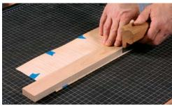
**Start with a straight edge.** After taping a couple of pieces of veneer in a stack, use a veneer saw and an MDF straightedge, with sandpaper stuck to the bottom, to cut one edge straight. Start with a light pass, and then bear down a bit more as you go.
