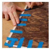
**Tape across the joints.** Pull blue tape across the miter joints, and across the all the edges. Stretch and pull the tape as you apply it.
