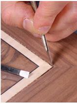
**Square the corners by hand.**Be careful not to rout too far, then finish up the corners with a narrow chisel and scalpel.
