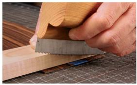
**Three good edges.** This time you need to cut the two long edges of the stack parallel before trimming one end square. These crosscuts want to tear out at the near end, so make a small reverse cut there before each pass.
