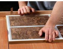
In the bag. After laying up the panel (left), you'll need to trim it. To get a first reference edge straight and flush with your banding, you can shim the panel on a crosscut sled (above). Then line up a framing square with that edge, using it to set up a straightedge and router on an adjacent edge. The tablesaw can take over from there.
