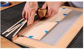
**Simple jig.** Make a cutting board as shown, plus a hardwood cutting guide the width of your desired bandings. Hold the guide and the veneer firmly against the stop on the cutting board. Cut enough banding to go around your panel, plus a few extra pieces.
