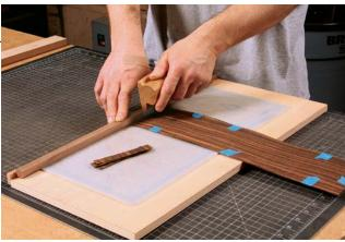
**Back to the cutting board.** Starting at the square end, cut as many strips as you need. As before, make a series of light passes for each cut, with a short reverse cut before each pass.
