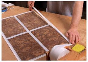
**Veneer tape next.** Remove the blue tape from the show face, and replace it with <sup>3</sup>/<sub>4</sub>-in. veneer tape. Then throw the sheet under a piece of MDF to stay flat. When it's dry, flip the sheet and remove the blue tape on the glue face.
