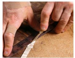
**Scarf the banding.** Stringing can have butt joints, but where the 2-ft.-long bandings come up short, use an angled cut to hide the joint. Just overlap the pieces, line up the grain, and use a scalpel and steel ruler to cut through both.
