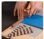
Crosscut your bandings. After squaring one end of the sheet, use the banding jig again. Cut tape-side-up, and make more than enough strips for the job.
