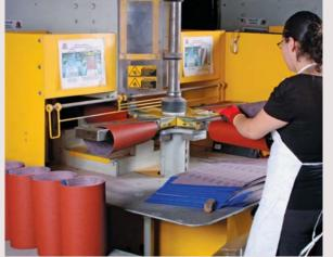
Belts begin as sheets. Wide sheets, with their ends cut on the diagonal, are wrapped around a form and heat is applied to glue the seam.
