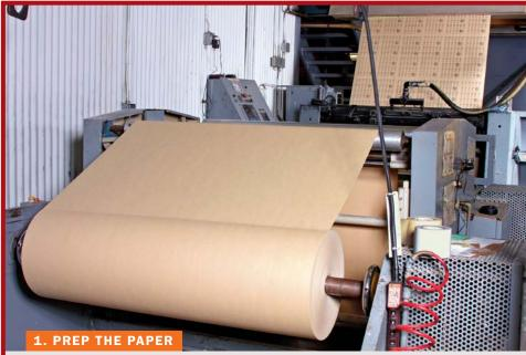
**Start with a blank roll.** Sheets, disks, or belts all begin life as a large roll of backing material. The first step is to print on the back what the product will be.
