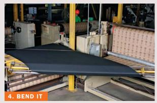
Micro-fractures. The stiff roll of sandpaper is bent back and forth at 90° and 45° to make it more flexible and to prevent it from cracking the first time you try to bend it.
