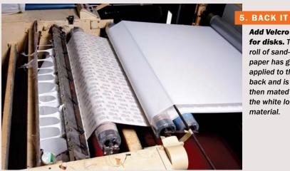
**Add Velcro** for disks. The roll of sandpaper has glue applied to the back and is then mated to the white loop material.
