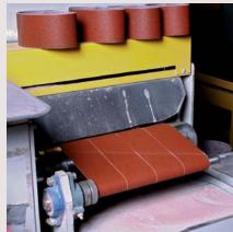
One loop equals four belts. The abrasive cylinder is spun across fixed knives to create four sanding belts.
