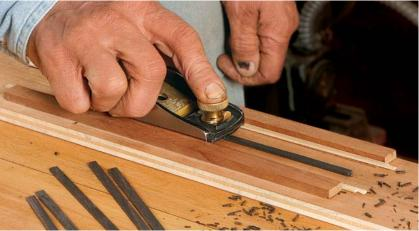
**Plane to thickness.** When thicknessing small ebony parts, Hack prefers hand over machine. He often uses a jig to ensure that all parts are uniform. It's simply a piece of plywood with thin runners that the plane rides on. A brad in front works as a stop.
