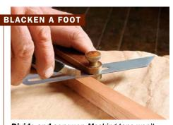
**Divide and conquer.** Masking tape won't block the dye from spreading. Instead, knife a fine line to divide the sections (above). Use a chisel to further define it (below), but don't press hard—a gentle touch will do.
