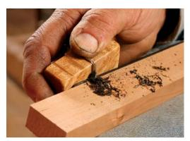
**Shape with a scratch stock.** Machines can cause wicked tearout on the brittle ebony, so Hack uses scratch stocks to shape the material. Here he shapes a bead applied to a door frame.
