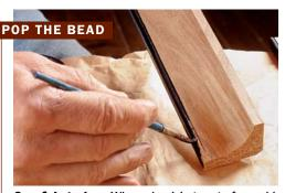
**Careful strokes.** When ebonizing part of a molding, such as this bead, it needs distinctly defined transitions. Otherwise, the dye will roam. The black bead on this crown adds a delightful contrast, breaking up the broad butternut surfaces.
