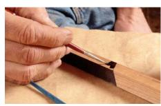
**Stay within the lines.** Use a fine paintbrush to apply the dye right up to the knife line. A wider brush can be used in the larger area.
