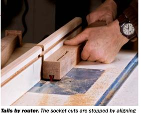
registration marks on the leg and fence (above). After cutting the tail at the same bit height (right), saw away the bottom ½ in. to fit the socket.
