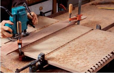
**Rout stopped dadoes for the vertical dividers.** Clamp the top and bottom pieces together at the back edges to rout both pieces at the same time. If your guide rail is square to the pieces, the dadoes housing the top and bottom of each divider will be perfectly aligned.
