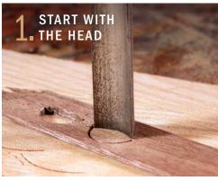
Transfer the layout to the door. After marking the location for the overall inlay, hold the workpiece in place to trace the outline of the head. Then tap with the gouges to incise the profile.
