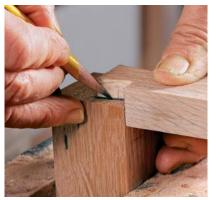
Tails by hand. Saw and pare the tail, then saw away half the thickness to create a lap on the bottom side of the joint (left). The lapped dovetail rests securely on the mating piece (above), making it easy to transfer the layout.
