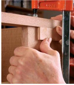
**Set it in place.** With the aprons and lower rail already glued up, set the front assembly in place. The aprons are simply edge-glued to the legs and top rail. Use a spacer (above) to dial in the location.
