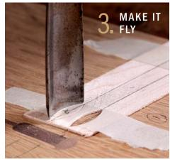
Step saver. With the veneer taped to the workpiece, chop through the veneer to create the inlay piece and mark its mortise at the same time (left). Then finish chopping the mortises. After the wings are in (below) and dry, plane and sand the veneer flush.
