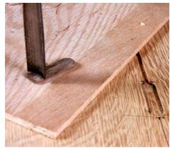
Mortise for the body and tail. Guide the router along a fence for a straight cut. Use a 1/2-in.-dia. bit for the body and 1/8-in.dia. bit for the tail (above). Use the same gouge that created the bottom of the head to cut a matching curve in the top of the body veneer (left).
