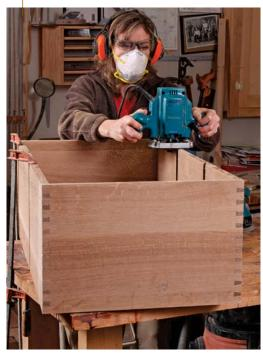
Rout the rabbet for the back and install the dividers. Hiller uses a %-in. rabbeting bit, set for a cut that is 5/16 in. deep. When skipping past the divider dadoes (above), be careful to keep the bearing from diving in. Tap the uprights home until their front edges are flush with the front of the case (right).
