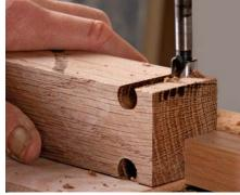
Shape the foot first. Hiller creates the sharp curve at the top of the foot by drilling out the cuff on all four sides with a 1/2-in. Forstner bit buried only partially in the wood.
