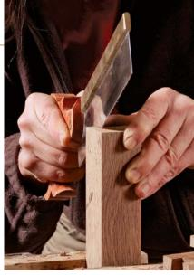
Saw and chop the socket. Align the saw with the layout lines and angle the blade downward as shown to cut as far as you can. Then chop and pare with a chisel to finish the socket.
