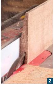
**Three angled cuts create the crown.** Hiller starts with a throughcut, running the stock on edge past the angled blade to create the crown's top rim (1). An angled cut along the opposite edge creates one side of the angled rabbet (2). And a shallow angled cut frees the waste (3).
