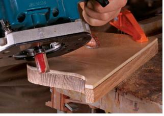
**After the bandsaw.** Use a bearing-guided router bit to trim the rough-cut curves on each apron flush with a plywood template (above). Hiller uses a hollow-chisel mortiser to make the mortise for the lower rail (right).
