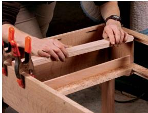
**Guides, then kickers.** Glued to the side of the drawer runners, the guides keep the drawer aligned in its opening (above). Install the kickers next; they keep the front of the drawer from tipping downward as it opens. They tenon into a groove in the top rail (left) and are screwed to a support block at the back (below).
