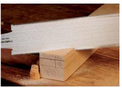
**Mortise first, then the tenon.** Drill the mortise and square it with a chisel, then saw away the sides to reveal the tenon's cheeks. Use a shoulder plane to clean those faces to the line.
