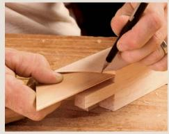
**Creating a profile.** Cut the desired profile on a piece of scrap, then transfer the shape to the stile. Mitering the ends of the scrap makes the transfer easy.
