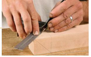
**Mark the bottom shoulders and 45**  $^{\circ}$  **miters first.** Start the miters about  $\frac{1}{26}$  in. from the end of the workpiece to let the tenons protrude.
