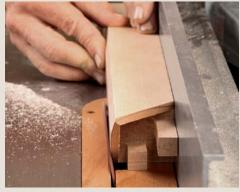
**Rough the shape at the tablesaw.** Rip the facets first, then fine-tune the shape with a handplane. Reassemble the joint and trace the profile from the stile onto the rails.
