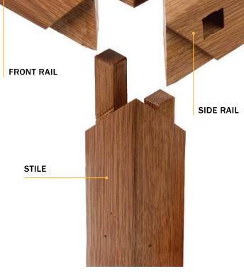
start to finish. However, it's worth mentioning that because the three parts of each joint are so different, in an actual project I lay out all the like pieces, move on to the next set of like pieces, and then lay out the last set. I do the same with the construction. I cut all the stiles first, then I cut all the mortiseonly rails (side rail, above), and then the rails with one tenon and one mortise (front rail, above).
