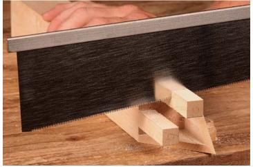
**Cut one tenon short.** Finish by cutting one of the tenons short to accommodate the tenon that will come in from the rail.
