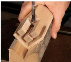
**Get rid of the back tenon.** With the front tenon gone, you have access to the back one. Drill between the two side tenons to remove it. Clean up the bottom of the joint with a chisel.
