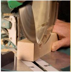
**Two mortises and a miter.** Use a drill press to remove the bulk of the mortises, and then chop to the lines with a chisel. Then use a chopsaw to cut the miter. Hunter cuts just outside the layout lines and then shaves right to the line with a handplane or chisel.
