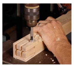
**Remove the front tenon.** Use a Forstner bit in the drill press to remove the section of the tenon that you wouldn't be able to reach with a handsaw.
