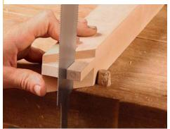
**Finish up the tenon.** Again with a handsaw followed by a chisel, cut away the remaining waste to leave the tenon.
