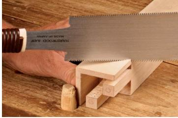
**Outside miters are easy now.** Cut the two mitered shoulders with a handsaw, then shave right to the line with a shoulder plane.
