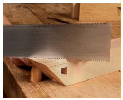
**Cut the mitered shelf.** Use a handsaw to cut the ¼-in.-deep shelf that will accommodate the mitered laps of the stile. Clean it up with a shoulder plane.
