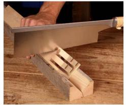
**Follow up with a handsaw.** Carefully cut off what remains of the front tenon.
