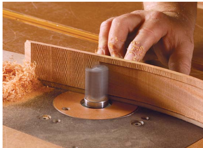
Trim the top edge. Attach the master template to the top edge of the molding and use it to guide a flush-trimming bit to clean up the top edge. Raise the bit to finish the job.
