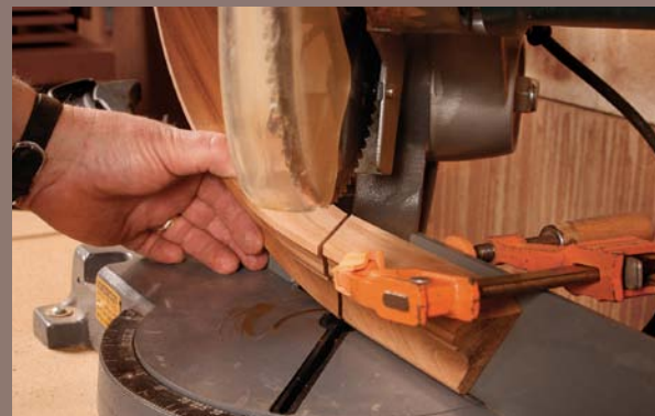
Cut the miter. Clamp both ends of the molding to the chop-saw's fence and then cut the miter. The left clamp is behind the author's hand.
