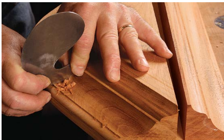
Blend and smooth with a scraper. A gooseneck scraper is ideal for cleaning up the different parts of the profile.
