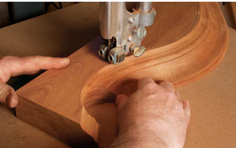
Cut out the molding. Bandsaw just outside the line that you drew before cutting the profile (see p. 75).
