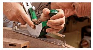
**No gap.** On outside curves, set the gap close to zero, but always feel free to adjust on the fly to improve the action.
