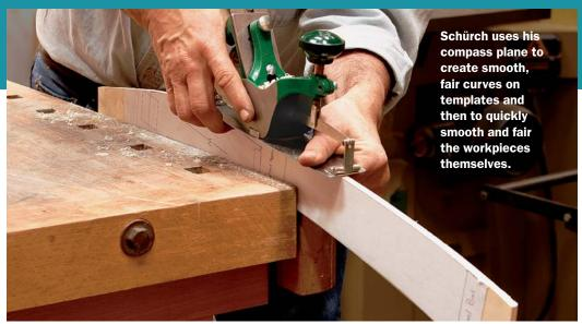
**Making templates.** After laying out his curves on paper, he glues that to template stock and planes to the line. Where a sander would leave a bumpy surface, the compass plane creates smooth, flowing curves.
