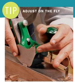
As the curve changes and the plane stops making shavings, the Stanley design makes it easy to fine-tune the sole between strokes.
