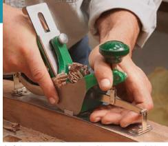
**Quicker, shorter strokes.** Plane more quickly than you would with a normal bench plane, with shorter strokes of 6 in. to 12 in. And focus the pressure on the front of the sole (above). On the return stroke, tip the plane upward (right) to avoid dulling the exposed blade.
