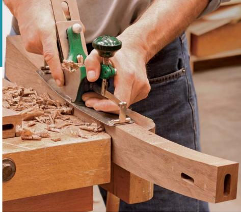
**Outside in.** With all curves, always plane from high to low to work with the grain and avoid tearout. On concave curves, this means planing from the ends toward the center.
