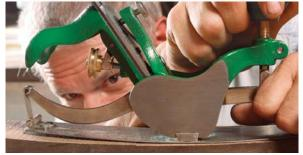
**Leave a gap.** Pressing the plane forward, adjust the sole for a ½2-in. gap between the back of the sole and the work.
