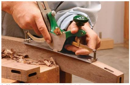
**Inside out.** Work from the center outward, and whether concave or convex, try reversing direction if you are getting tearout.
