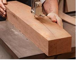
**Roughing out.** Template routing doesn't work well on thicker workpieces, so Schürch lays these out with the template (left) and then bandsaws close to the line (right).
