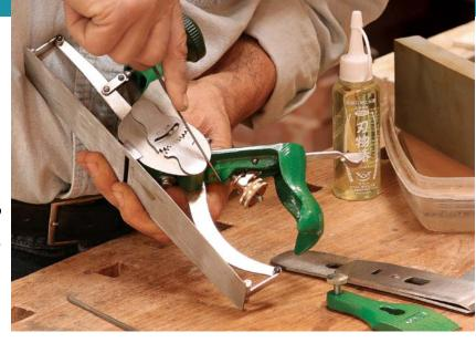
plane, make sure that both sole plates are riveted cleanly and securely to the plane body, and that neither is bent or twisted from the plane being dropped. Also, there should be little-to-no play in the adjustment gears or the arms that connect the sole to the plane body, and no missing or cracked parts.
