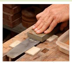
**Stone the bottom.** Adjust the sole flat, lock down the plane using a vise and blocks as shown, and sand the area around the mouth flat, finishing with honing stones.
