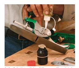
**Lube job.** Use a light oil like camellia to lubricate the moving parts, and to protect all of the exposed steel in general.
