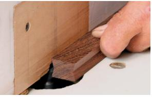
**Rout the V.** Mark the midpoint of the stock and set the bit height so that the cut doesn't touch the top half. With the top and bottom of the dovetail cut, you may be left with a thin line down the center that can be snapped off by hand.
