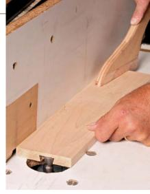
2. Finish at the router table with a dovetail bit. Use measurements from the full-scale drawing to locate the fence.
