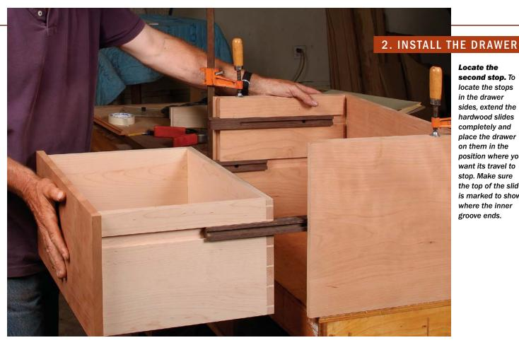
Locate the second stop. To locate the stops in the drawer sides, extend the hardwood slides completely and place the drawer on them in the position where you want its travel to stop. Make sure the top of the slide is marked to show where the inner groove ends.
