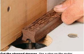
**Cut the stopped grooves.** Use a stop on the router table fence and pivot the workpiece up when you reach it. Remember that the grooves are on opposing faces and start at opposite ends of the slide.
