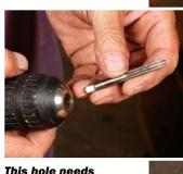
threads. The setscrew that serves as the stop in the case side can't cut its own threads, so you'll need to cut them using a standard ¼-20 NC tap, available at Amazon.com and online hardware dealers. Follow up with a ¼-20 bottoming tap to thread the hole all the way to the bottom.
