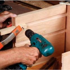
**Drill for the first stop.** Mark the case side at the point where the access hole falls when the slide is inserted a little more than a quarter of the way into the case. Use a guide block as shown to keep the drill straight; a piece of tape marks the bit depth. A 3/16-in. brad-point bit centers easily and cuts cleanly.
