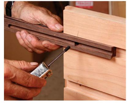
Install the set screw. With the slide in the groove, insert the screw through the access hole and into the threaded hole in the case. Continue turning the screw until the slide moves freely in its slot but is halted by the stop.
