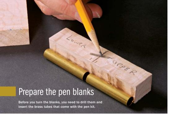
**Lay out the blank.** Each section should be a little over 1/8 in. longer than its respective tube. Label the parts and mark their relationship for grain continuity.
