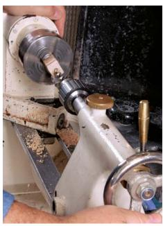
**Drilling on the lathe is easiest.** Cut the parts to length, then secure each blank in a pen-drilling chuck or a conventional four-jaw chuck (shown).
