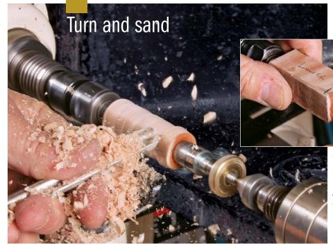
Round it. Insert the correct size bushing (above). Use a roughing gouge to turn the square blank round (left).
