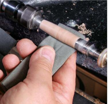
sand it. Smooth the wood with sandpaper to 800 grit, then switch to Abralon cushioned abrasive pads and go up to 4,000 grit. Each grit needs to be applied for a few seconds only.
