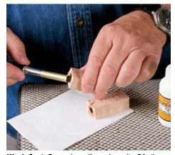
**Work fast.** Spread medium-viscosity CA glue on some glossy paper. Roll a tube in the glue and then use either a dedicated insertion tool or a nail punch to push it into the blank.
