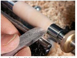
**Refine it.** Use a Spindlemaster (left), or if you are comfortable with it, a skew chisel to bring the blank to its final size and shape. To bring the ends of the blank flush with the bushings, use the skew (right) or Spindlemaster like a scraper.
