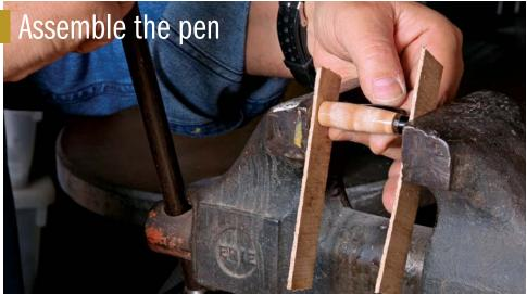
Any vise works. You can buy a pen press to assemble the pen, but as long as you protect the components, a metalworking (or woodworking) vise works almost as well.
