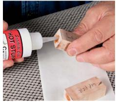
**Stabilize the blanks.** In any natural wood (as opposed to impregnated or stabilized woods sold for pen turning), you should "size" the holes with thin cyanoacrylate (CA) glue.
