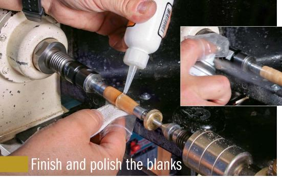
A super finish. Apply medium-thick CA glue to the turning blank as you spread it with a paper towel. Wear a disposable glove or wrap your finger in a plastic bag. Use an aerosol accelerator to instantly cure the CA finish (inset).
