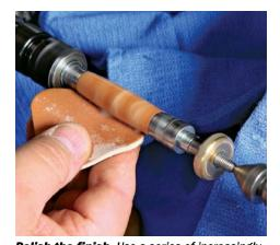
Polish the finish. Use a series of increasingly fine abrasive pads designed for acrylic to polish the finish.
