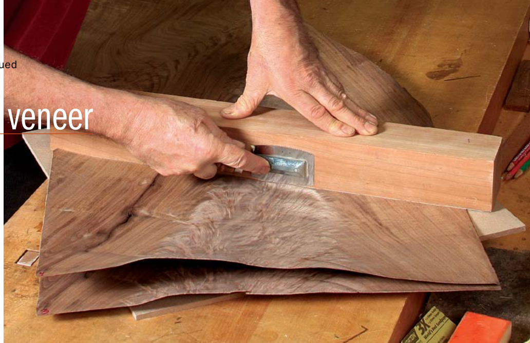
Rough out the veneer. With the two sheets for a book-match stacked and aligned, use a veneer saw and straightedge to rough out the pieces. The straightedge must be wide enough to register the veneer saw fully.
