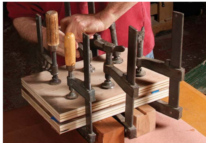
Keep an even keel. The panel should see even pressure across the cauls, so using numerous clamps is advantageous even on a small panel. Give the panel 24 hours to cure before removing the cauls.
