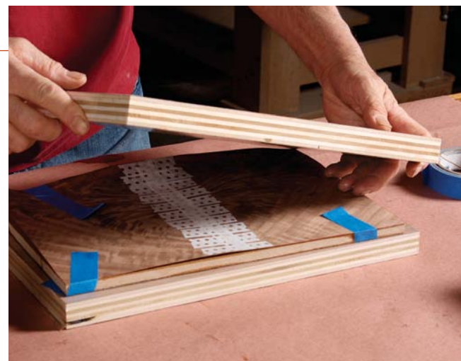
Roll out the brown carpet. Roll a healthy coating of liquid hide glue on the substrate for the panel (left). The coating has to be even and full to avoid dry spots. After both sides are loosely taped in place on the substrate, put the panel in the cauls for clamping (right).
