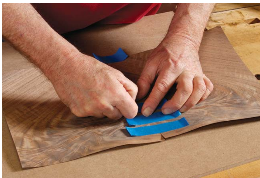
Tape brings it together. After lining up the grain for the match, stretch blue tape from one side to the other to bring the seam together tightly. Folding the ends of each strip makes removal much easier.
