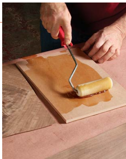
Roll out the brown carpet. Roll a healthy coating of liquid hide glue on the substrate for the panel (left). The coating has to be even and full to avoid dry spots. After both sides are loosely taped in place on the substrate, put the panel in the cauls for clamping (right).
