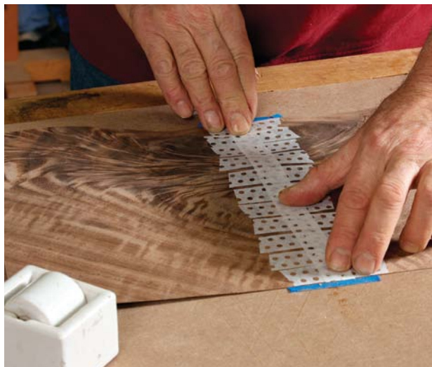
Tape brings it together. After lining up the grain for the match, stretch blue tape from one side to the other to bring the seam together tightly. Folding the ends of each strip makes removal much easier.
