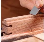
Notch for the handle. After marking out the notch (above), Mays removes most of the waste at the bandsaw, then cleans up the cuts at the router table (right).
