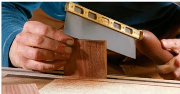
Saw the pins. Mays uses a saw that has no teeth at the front or back of the blade (\$139, Glen-Drake Toolworks: play-glen-drake .com). The design lets the saw build momentum before
