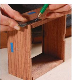
**Two edges of the lid rest on the sides.** To make room, trim those two box sides flush with the bottoms of the rabbets on the adjacent sides.
