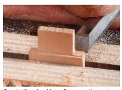
**Create the shoulders.** Saw away the waste on each end of the tenon. Then pare the excess flush.
