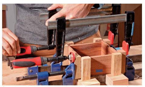
**Clamp thoroughly.** Mays applies pressure in both directions on each joint, checking for square and adjusting the clamps as needed. She uses cork-faced cauls to accommodate the protruding tails and pins.
