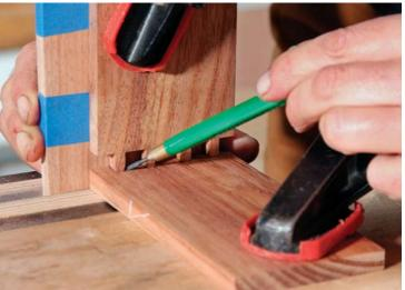
Transfer the layout. Clamp the pin board to a piece of wide stock held in the vise. Blue tape on the backer board shims the pin board forward so it aligns with the scribed baseline.
