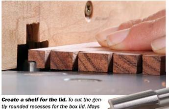
uses a high-speed-steel straight bit (right)
