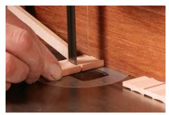
**Cut the handles from the blank.** After ripping two rows of handles from each blank, crosscut the individual ones free from each row.
