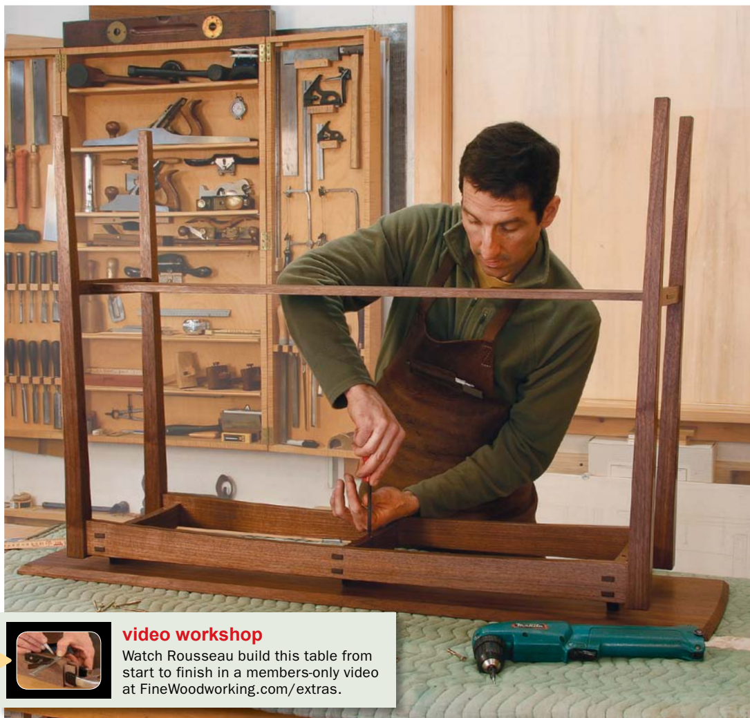
Inverted at the end. After gluing the legs to the aprons and preparing all the parts for finish, Rousseau attaches the top with three screws through each under-rail.
