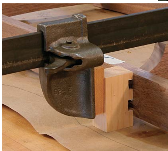
Clever clamping blocks. Rousseau makes custom clamping blocks that accommodate the proud through-tenons. He faces them with packing tape to keep glue from sticking.
