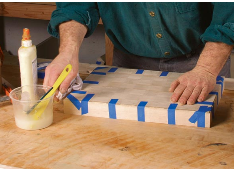
Begin veneering at the top. Liberal amounts of blue tape hold a veneer sheet securely in place on the top of the carcass.
