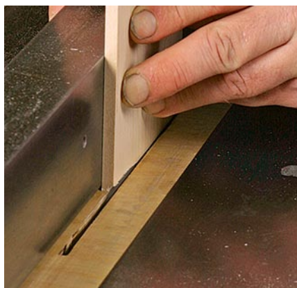
Small, simple joints. Use the tablesaw to cut the joints for the box carcass. Begin by making a \frac{1}{8} -in.-deep dado in the long side pieces (left). With the same fence and blade-height settings, cut the mating rabbets in the short sides (right).
