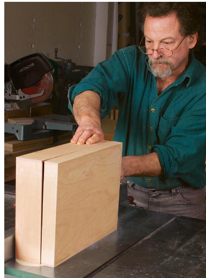
Open the box. This is the final step in assembling the box carcass. Progressively deeper cuts on the tablesaw separate the bottom section from the top.
