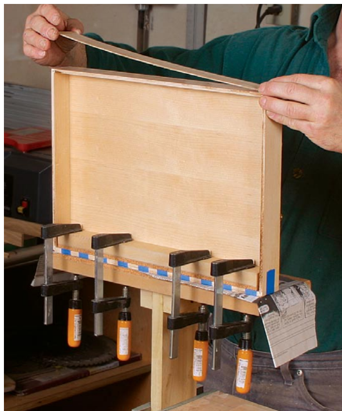
A box-sized caul. The top is clamped in an antique book press while the glue dries. A caul, made of layers of medium-density fiberboard (MDF) with cork padding on one face, provides even pressure. If you don't happen to own an antique book press, a pair of cauls and lots of clamps will do nicely.
