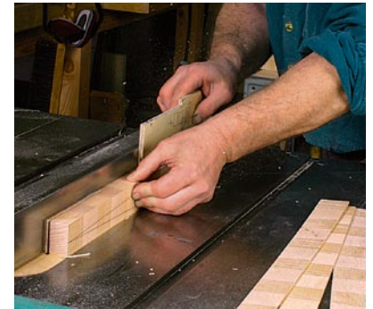
Block becomes veneer strips. Maple blocks are stacked so that the edge grain is alternately horizontal and vertical. Then they're glued and clamped in a simple fixture (left). Once completely dry, the glued-up block is ripped into strips ¼ in. thick (right).
