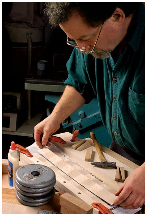
The second glue-up. Veneer strips are edge-glued a few at a time (left). Old newspaper keeps veneers from sticking to the gluing jig. The strips are staggered to create the checker-board pattern.
