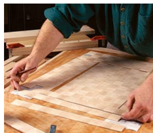
Spreading the sheets. Once the parquet panels have dried, lay them out and arrange side panels to match the grain pattern with the top panel.
