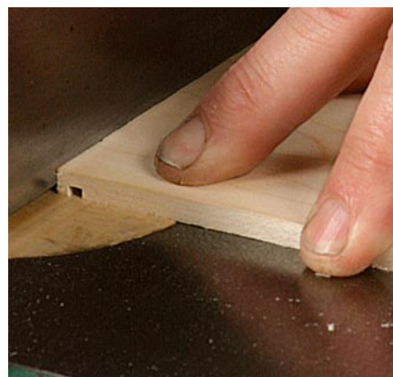
Small, simple joints. Use the tablesaw to cut the joints for the box carcass. Begin by making a \frac{1}{8} -in.-deep dado in the long side pieces (left). With the same fence and blade-height settings, cut the mating rabbets in the short sides (right).
