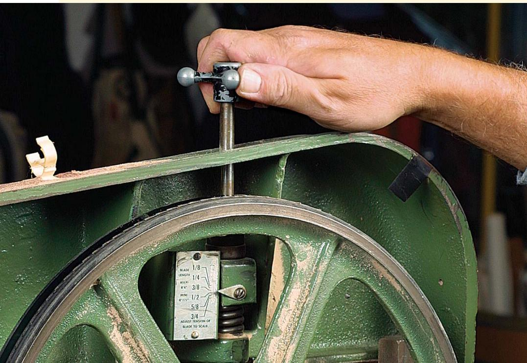
**Use less than the recommended tension.** For a 1/2-in.-wide blade, turn the tension gauge (above) to the setting for a 3/8-in.-wide blade. The first step in overhauling a bandsaw is to check the tires for grooves (right). If necessary, replace them.
