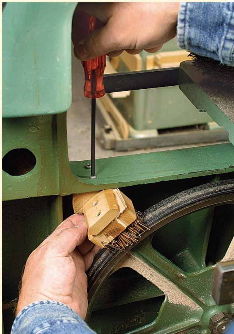
block to within the thickness of cigarette paper, or 0.001 in., of the blade. The Allen screw might pull the blocks in or out when they are tightened, so this process could require one or two attempts. With practice, you will be able to adjust the guides by eye, looking for the smallest crack of light between the blade and the guide blocks.
