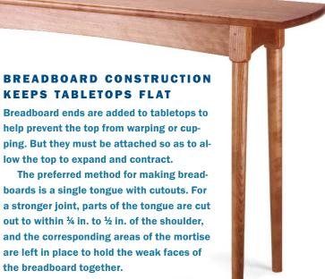
The trickiest part of construction is pinning and gluing the breadboard ends. I like to plane a slight (1/16-in.) concave bow into
