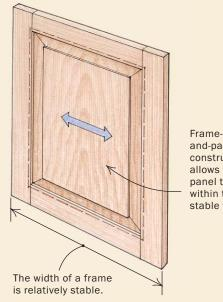
and-panel construction allows the panel to move within the stable frame.
