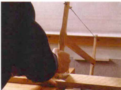
Crosscut with a bowsaw. Keep your wrist angled outward, and with a little practice, you'll be able to make square cuts.
