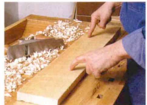
Check a board's flatness. Place your fingers on diagonal corners of the board. If the board rocks on the bench, move your fingers toward the center. When the board rocks no more, the high spot is between your hands.
