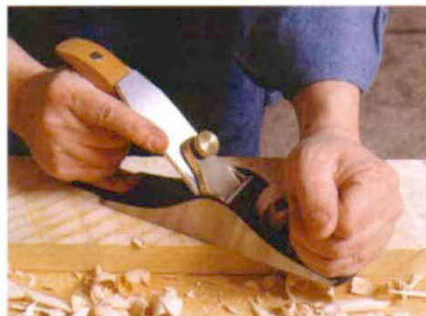
Scrub plane is for flattening. Using a scrub plane, with its radiused blade, work the board diagonally in one direction and then the other.
