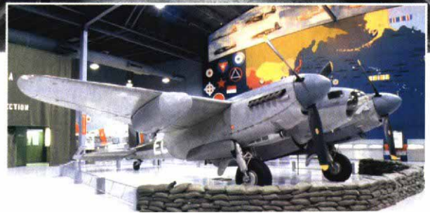
The "wooden wonder." This British-designed World War II plane, called the Mosquito Bomber, was constructed mostly from wood and bonded with urea formaldehyde glue, which had just been developed.
