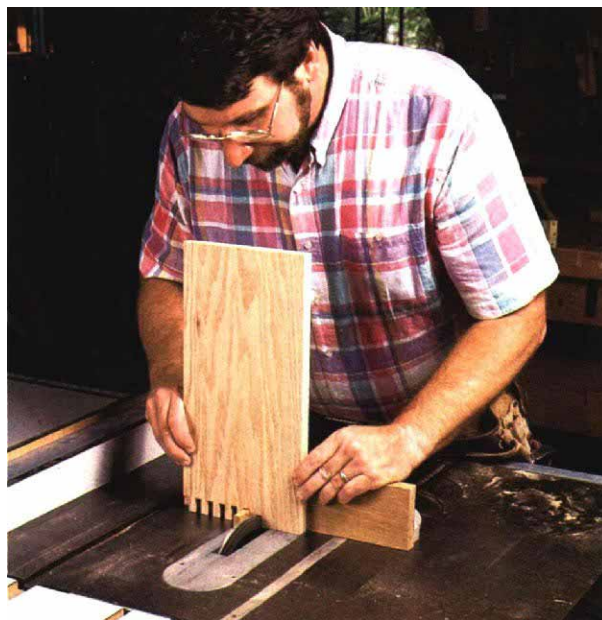
Finger-saving finger joints: Abram uses jigs, especially when a machine's guard has been removed for photographic clarity (or otherwise). To make tablesaw operations logical and safe, he builds jigs, for example, that ride in the saw's miter grooves, as shown here.
