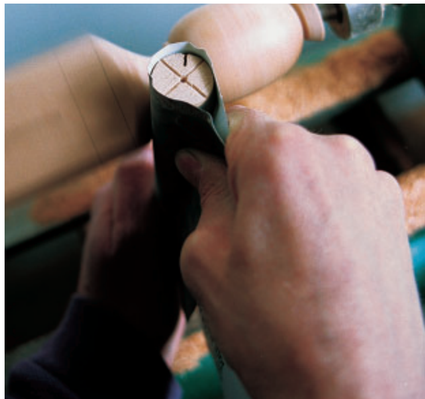
Photo F: Sand the transition from square to round using a sanding block so you don't blur the edges sanding by hand.
