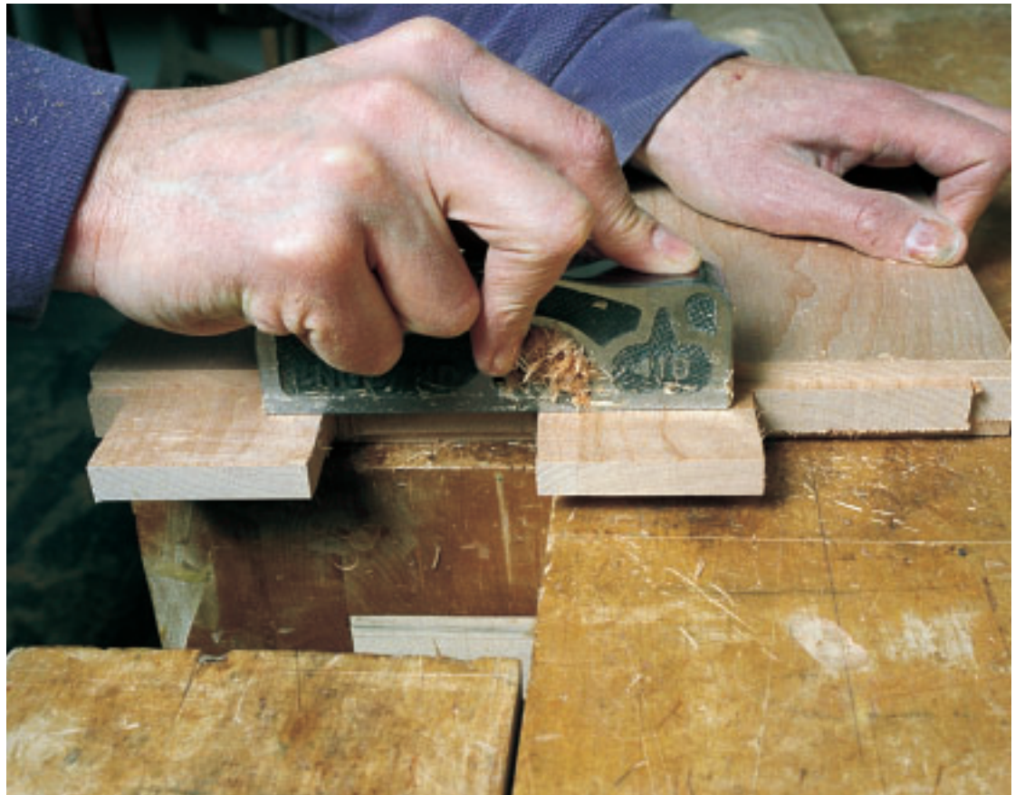
Photo H: Trimming the cheeks of the tenons to fit the mortises is easy with a shoulder plane. Note that you cut across the grain.
