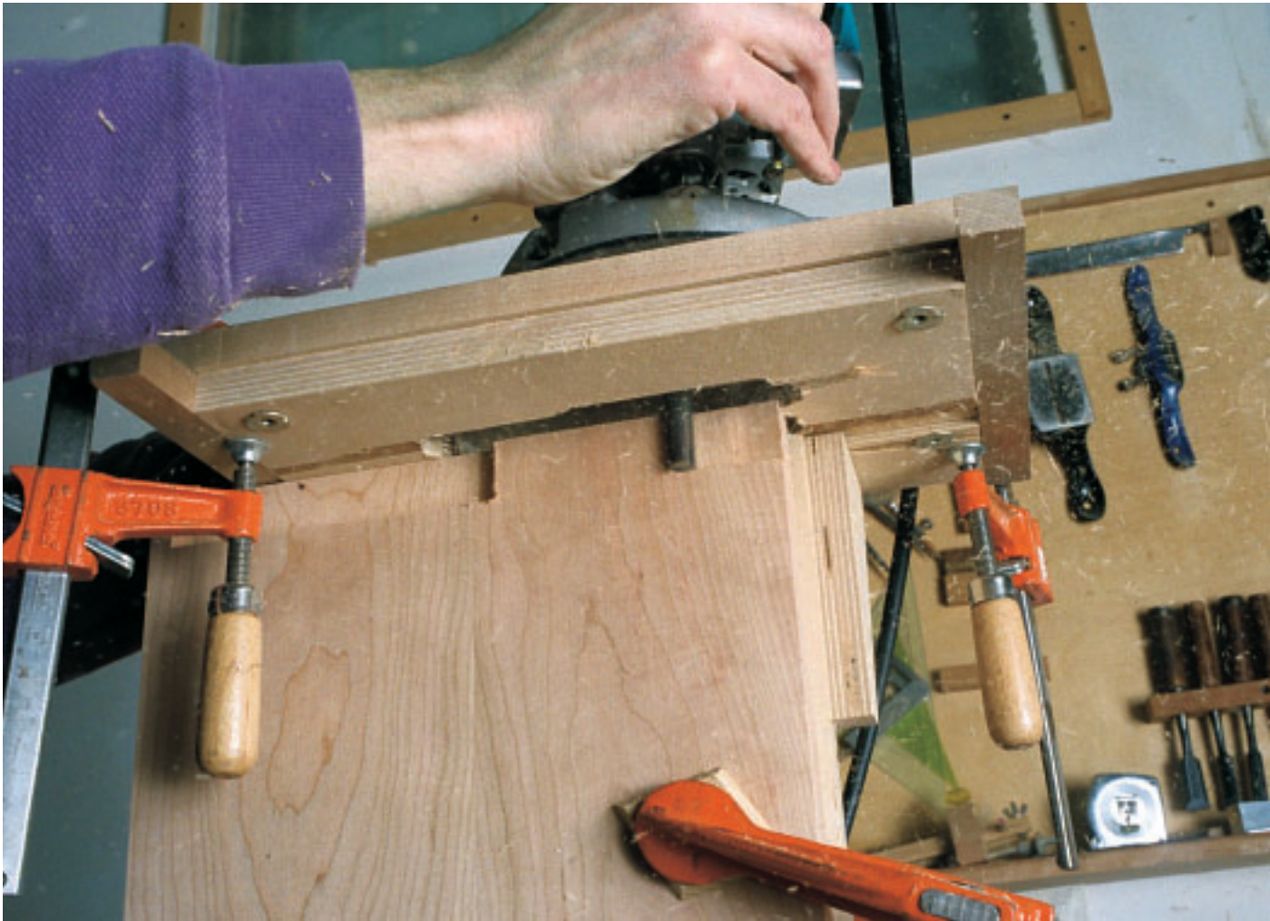
Photo A: One good way to cut the full-width tenons on the headboard and footboard is with the tenoning jig on p. 24 and a 4-in.-long router bit.
