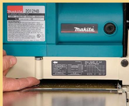
**How big a bite?** There are different ways to determine how much material will be removed. Delta's "Blade-Zero" device (left) pops up when the cutterhead is even with the top surface of the board; from there the depth of cut is set by turning the crank a measurable amount. On the Makita (center) a loose pin moves with the cutterhead against the top of the stock, giving a visual idea of how deep the cut will be. Other models have depth-of-cut indicators that give an exact measurement (right).
