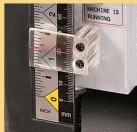
**Digital display, mechanical stops, or a simple scale.** All these devices indicate the thickness of the material. The Craftsman 21759 (right) has a digital readout that is extremely accurate. Scales (above) and stops are much less precise.
