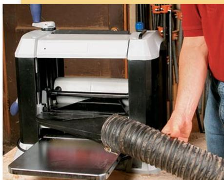
**Helpful new features.** The chute on the Delta (above) flips to allow the hose to connect to either side. The Craftsman 21759 (right) and DeWalt 735 blow their own chips into almost any container, without a dust collector attached.
