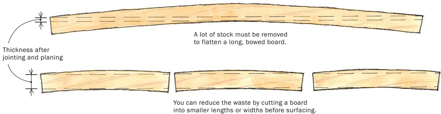
defects such as knots, sapwood or checks. Use a chopsaw or hand-saw to rough the stock to length, removing any checked or cracked areas on the ends. Next, rough your stock to width. This can be done in a variety of ways. If the board is badly crooked, you may need to snap a chalkline on it and bandsaw to the line. Otherwise, run one edge over the jointer or handplane the edge to level it out. Now you can rip the board to rough width.
