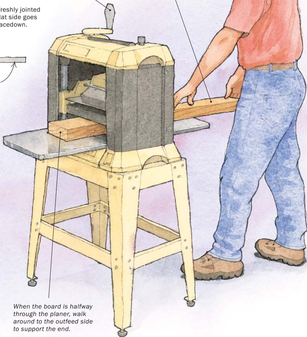
dency to snipe at the beginning and end of a board. Plane all of the boards down to thickness, leaving them a hair oversize to allow for removing the milling marks. These marks are not a decorative effect.
