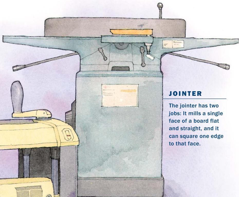
Armed with both, you can flatten boards to any thickness
