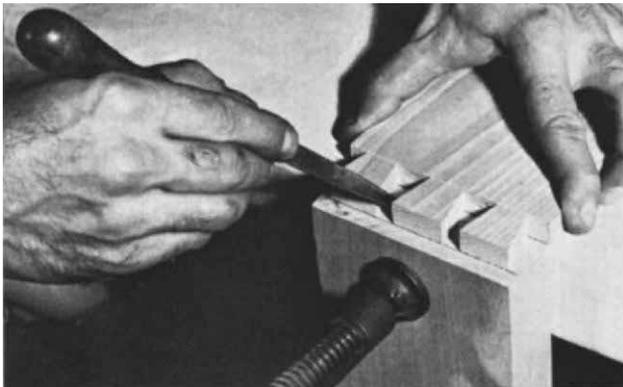
side over it. Be sure inside surfaces are towards the inside of the corner. Line the edges of the boards up, and position the ends of the tails exactly at the marking gauge line. This positioning is critical. If it is not done accurately, it will result in gaps. Clamp or hold the piece securely and scribe the pins from the sides of the tails. The lines should then be extended
