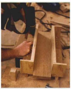
2. Use chair part to set jig. After securing one basepiece, the author snugs the other one against a side stretcher and screws it in place.
