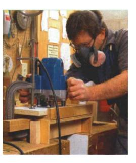
4. The depth of the mortise is controlled by the plunge mechanism on the router. The author secures stock to the jig with C-clamps.
