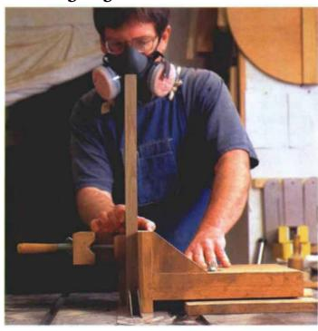
**Double-blade tenoning on the tablesaw**—With a custom-made jig, the author cut angled tenons for the side stretchers and side seat rails. Sawblades were set at a 4° pitch to the surface of the saw table and separated by a 1/2-in. spacer.
