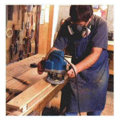
A plywood jig for shaping the back posts. A little time invested in this jig guaranteed that all back posts would be the same size and shape. A shaper with a rub collar works as well as a router.
