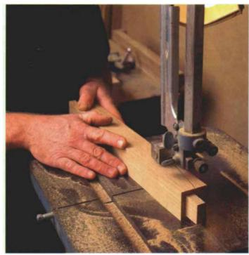
Cutting the curved back slats—Convex and concave cuts from 8/4 lumber yielded 7/8-in-thick slats, after the surfaces were scraped clean. These slats are the only curved pieces of the chair.
