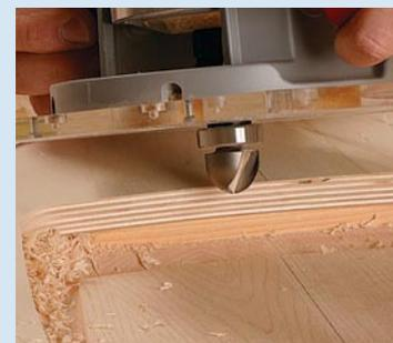
**If you need one, rout the juice groove next.** Use the first template to make an outside template, which will guide a top-bearing, roundnose router bit (top) or a router outfitted with a template guide.
