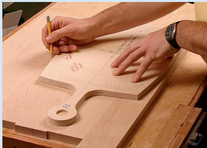
**Start with a template.** This lets you fine-tune the shape before cutting into your good wood. Trace the shape onto the stock.
