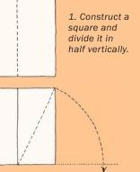
2. Draw an arc with a radius equal to the diagonal of one half of the square.
