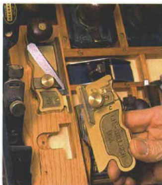
Fitting a tool. Odd-shaped tools, such as this side rabbet plane, fit into french cutouts in the shelf.
