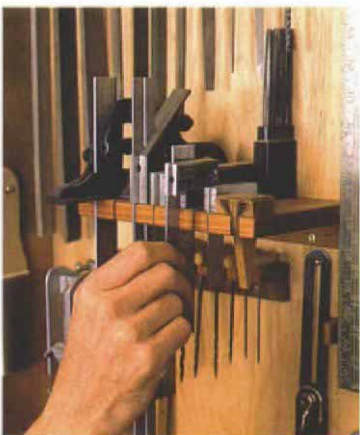
Shelved squares. Becksvoort's squares slide into sawkerfs cut on a small shelf, which takes up much less space than laying them out flat.
