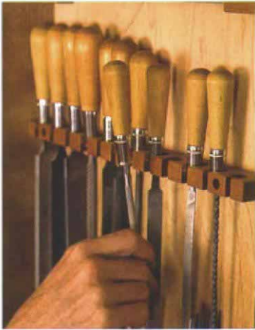
Simple is often best. Awls and screwdrivers rest in holes drilled into a small shelf.
