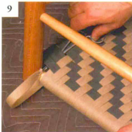
Surgical clamp reaches into tight spaces. It can be used to push or pull the tape. Doctors use this tool, so do fly fishermen. A clamp costs less than $10.
