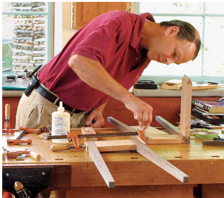
Assemble two sides first. If the splay angle is minimal, as in this case, there is no need to add wedges under the clamps.
