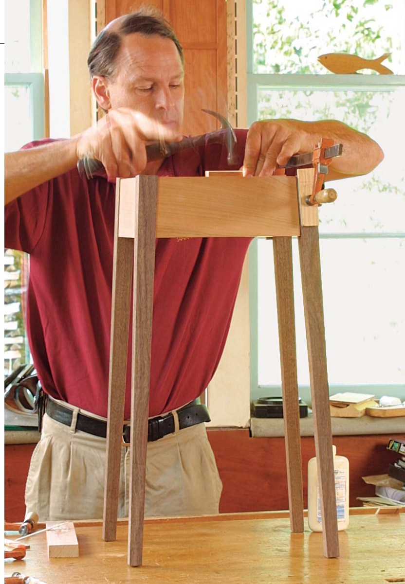
Glue in the front and rear aprons. Tap the aprons into their mortises with a hammer and block.
