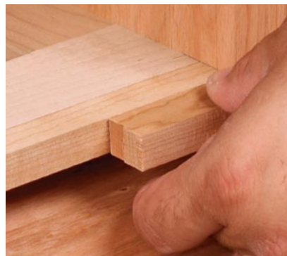
Glue, then shape. It's easier to glue oversize blocks to the frame and then shape them than it is to shape tiny pieces on the bandsaw and then try to clamp these irregular parts to the divider.
