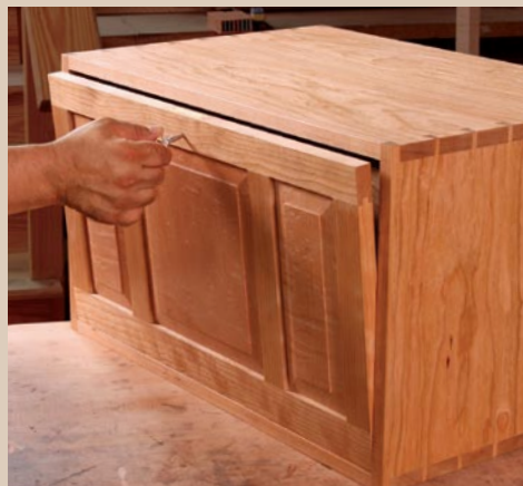
A secure lid. A lock mortised into the top edge and two pins on the bottom hold the lid in place.
