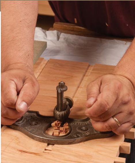
Hand tools complete the dadoes. Square the end of the dado with a chisel, and clean out the bottom with a router plane.
