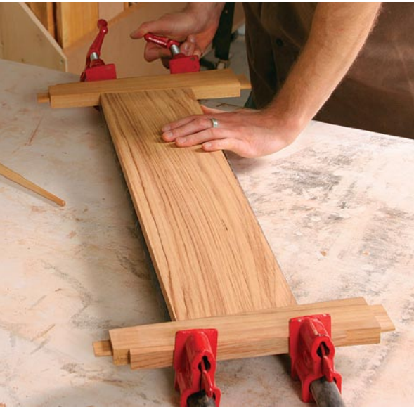
Glue the center rail to the center back splats. Jensen uses the cutoff pieces from the tapering process to create a square clamping surface (above). The tapered back splats, center rail, and crest rail complete the glue-up (right).
